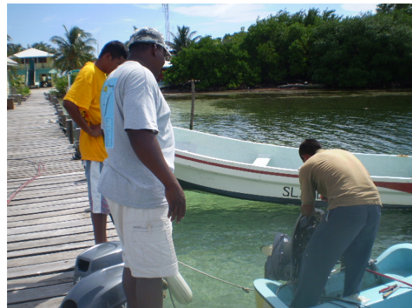
Figure 16. Staff changing control cables on boat engine
