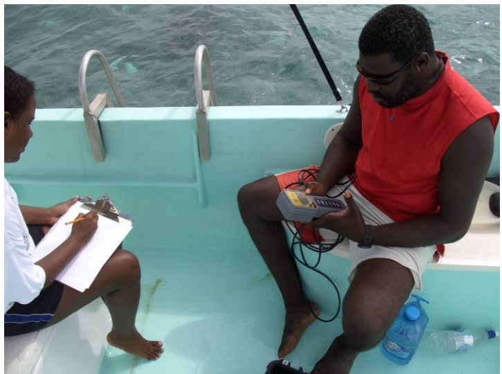
Collecting water quality parameters using a Yellow Springs Instrument (YSI) meter
